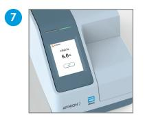
Record the result when it appears on the screen. Touch  $\checkmark$  to accept. The lid opens automatically.
