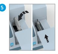
Insert the test cartridge with the barcode facing left. Close the lid manually to start analysing.
